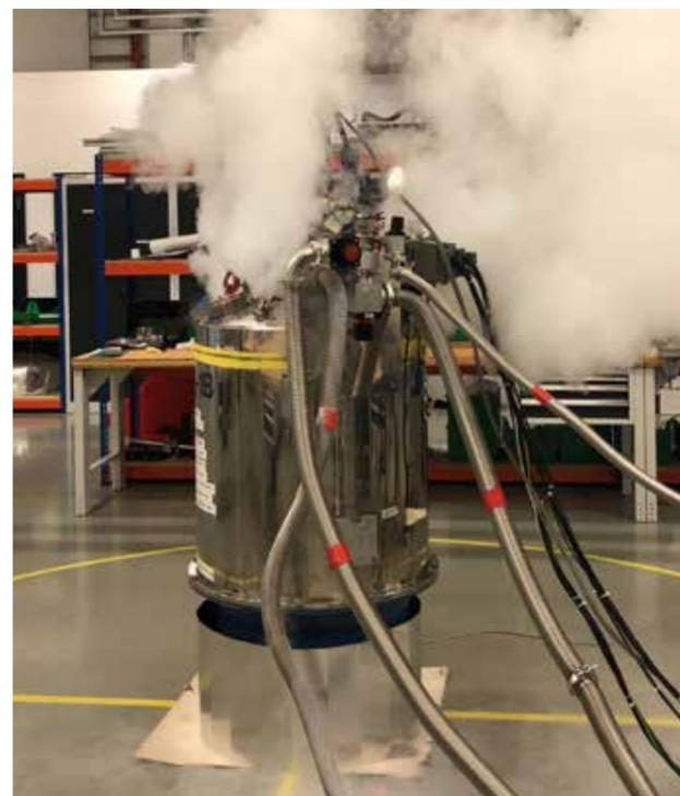
In November, the MSPS team successfully testing a dilution fridge in the sample environment workshop, achieving an ultra-low temperature of 27 mK. The Oxford Instruments dilution insert from HZB, tailored to fit within various sample environment devices, can be used with the 15 T magnet enabling users to subject their samples to high magnetic fields at extremely low temperatures. This capability is particularly valuable for experiments on the BIFROST instrument.
