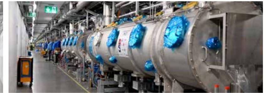
**Accelerator Tunnel:** The accelerator was commissioned with beam through DTL-4, the temporary shield wall removed, and the DTL-5 tank was installed as well as 13 spoke and 6 medium beta cryomodules. Repairs were conducted on the cryogenic distribution system (CDS) valve boxes and a second cool-down of the CDS showed that this work was successful.
