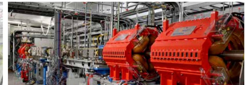
**A2T:** All technical components for the Accelerator to Target (A2T) beam transport system were installed, including the focusing magnets and correctors as well as the critical beam rastering system that will distribute the beam energy over each target segment.
