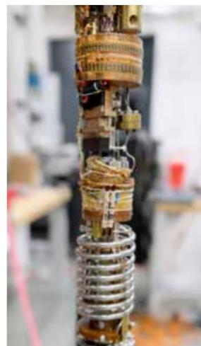
For the purpose of neutron experiments, the dilution fridge is constructed as a 'stick' on where the sample will be mounted at the very bottom. This stick can then be mounted on the neutron instrument, such that the neutrons pass through the sample. Here we see the inside of the dilution fridge stick in the ESS Sample Environment Lab.
