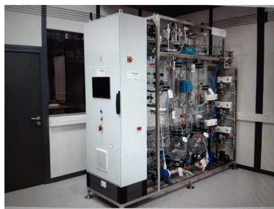
CO 2 Capture module ready to be assembled into the CO 2 LAB (EDF) Photo: BRGM
