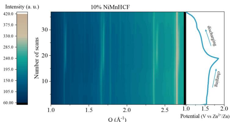
CERIC PhD candidate **Dr. Mariam Maisuradze, Prof. Marco Giorgetti** (University of Bologna) and colleagues followed the electrochemical behaviour of a partially (10%) nickel-substituted manganese hexacyanoferrate used as cathode material in a AZIB system, monitoring the structural modification of the material using synchrotron-based x-ray techniques. In particular, scientists exploited XAS and the powder x-ray diffraction (PXRD), both available at the CERIC Italian Partner Facility at Elettra.
