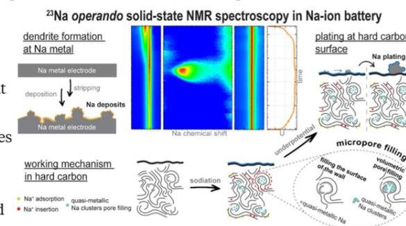
"We provided an in-depth analysis of the formation and composition of solid electrolyte interphase, understood and differentiated the sodium storage processes, and distinguished between Na plating and dendrite growth".
