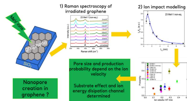
The findings coming from this systematic investigation enable custom-made production of nanoporous graphene using high-energy heavy ion beam for a variety of applications, including the development of nanomembranes for gas separation, sensors, or even separators Li-ion batteries and supercapacitors.
