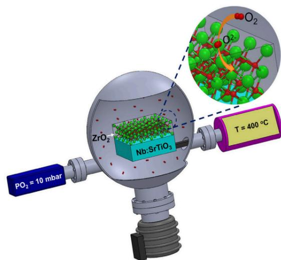
They then demonstrated through density functional theory simulations and by investigating the structural properties, chemical composition and ferroelectric properties of the films before and after an annealing at moderate temperature (400 °C) in an oxygen-rich environment, that oxygen vacancies are a key factor for stabilizing the polar rhombohedral phase and a possible source of ferroelectric polarization.
