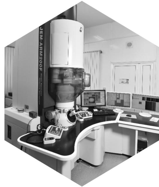
new EDS spectrometer on the JEM ARM200F atomic-resolution transmission electron microscope for qualitative and quantitative analytical investigations with high spatial resolution.
