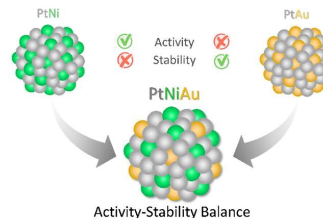
The optimal solution may lie in combining both approaches - using platinum alloys with transition metals to increase cost-efficiency while additionally incorporating gold for stability enhancement, and several studies on ternary Pt–Au–M catalysts have shown promising results. However, a deeper understanding of the underlying mechanisms and the detailed composition and distribution of elements in such complex alloys is essential for further progress.
