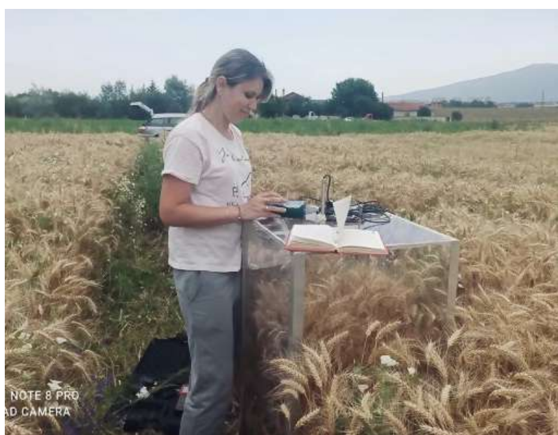
Figure 11: Measuring greenhouse gas fluxes (CO 2 , N 2 O) at Bozhurishte Open-Air facility using portable gas analyzers ALMEMO “MA2590-4” for determination of CO 2 and GASTiger 2000 for determination of N 2 O.
