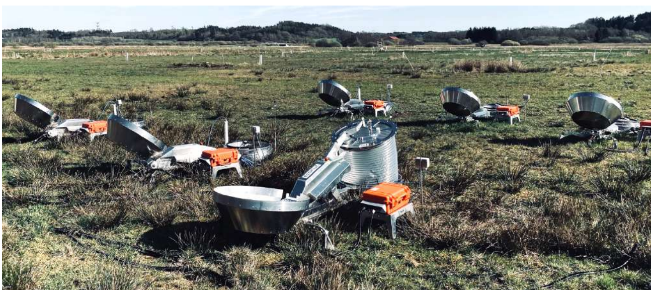
Figure 6: New technologies have recently been acquired at several facilities of AnaEE Denmark, including LI-COR eddy covariance towers and EcoFlux chambers from DMR as seen here at the Foulum facility.
