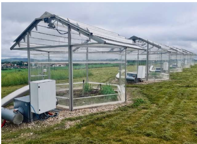
Figure 10: Experimental facility OTC Domanínek in 2023 after finished reconstruction. It is a fully automated facility, allowing manipulation of CO 2 , water and UV- radiation among other things, - allowing the evaluation of complex interactions of multiple factors.
