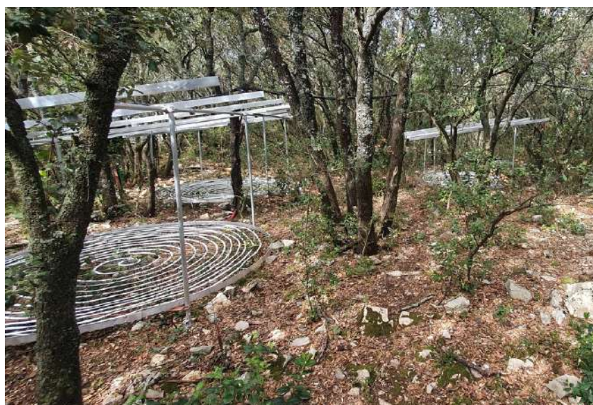
Figure 9: A new experimental set-up to manipulate soil temperature and rainfall in the forest understory at CNRS, Puéchabon open-air installation. The equipment was installed in 2023 and will be operational in 2024.
